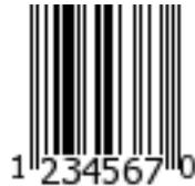
This barcode extends `Zend\Barcode\Object\Upca` (*UPC-A*), and inherits some of its capabilities; it also has a few particulars of its own. The first character of the text to encode is the system (0 or 1).
