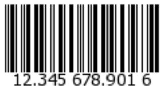
This barcode extends `Zend\Barcode\Object\Code25interleaved` (Code 2 of 5 Interleaved), and inherits some of its capabilities; it also has a few particulars of its own.
